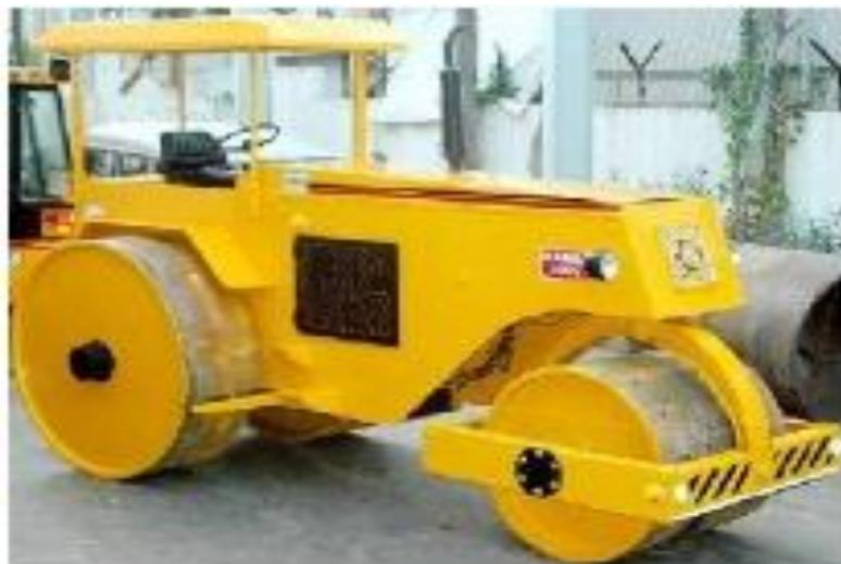
Gambar 2.2 *Three Wheel Rollers*
