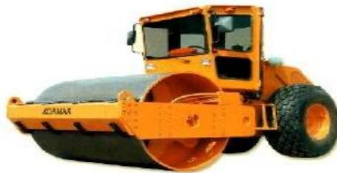
Gambar 2.4 *Vibration Roller*
