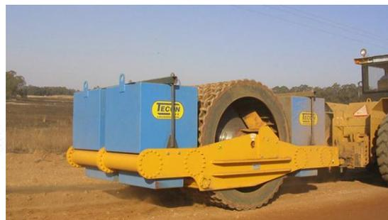
Gambar 2.5 *Mesh Grid Roller*
