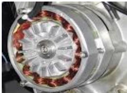
**Gambar 2.8 Stator (IE3 energy-saving motors)**
