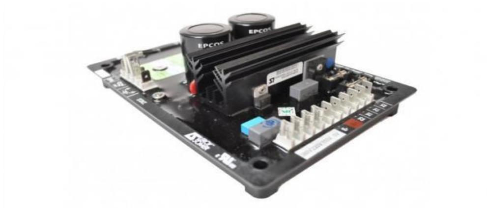
**Gambar 2.18 Automatic Voltage Regulator ( AVR )**
