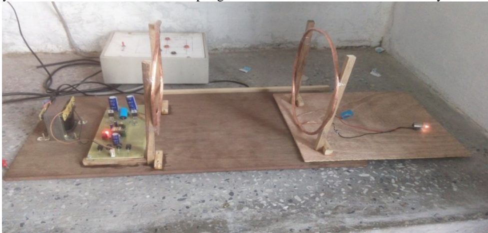
Fig 6: Designed model of the carried out experiment, the distance between the transmitter and the receiver coils was measured i.e. 35 cms with an efficiency of 82.8%.
