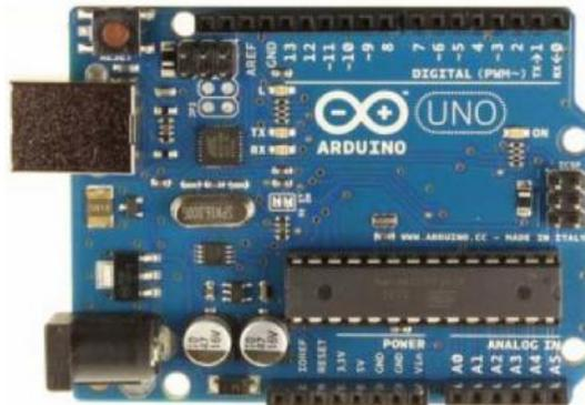
**Gambar 2.7** *Board* Arduino Uno
