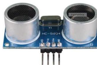
**Gambar 2.3 Sensor Ultrasonik HC-SR04**
