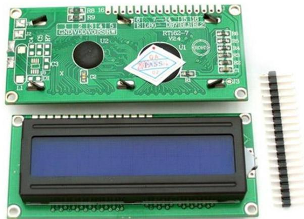
**Gambar 2.5** LCD 16 x 2
