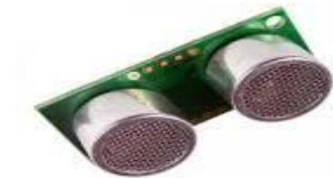
**Gambar 2.2 Sensor Ultrasonik Devantech SRF04**
