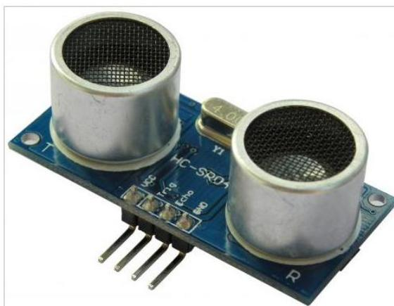
**Gambar 2.20** Gambar Sensor Ultrasonik HC-SR04
