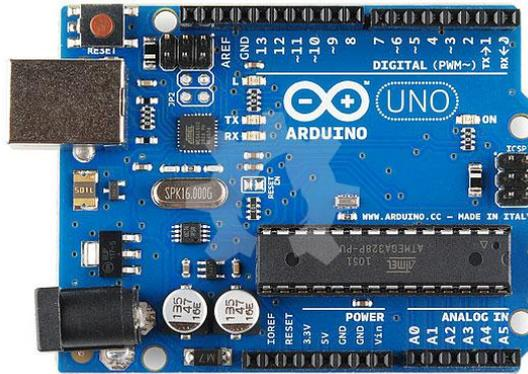
**Gambar 2.4** Papan Arduino Uno
