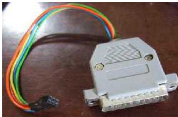
Gambar 2.12 Downloader Port Paralel model koneksi standar ISP 6 pin
