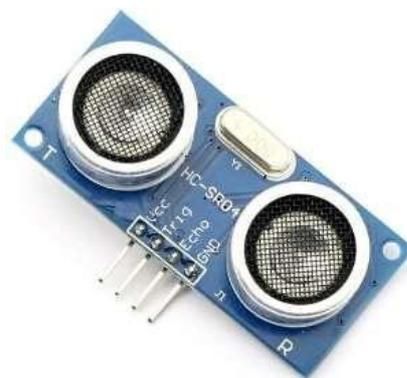
**Gambar 2.14. sensor ultrasonik HC-SR04**
