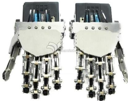
**Gambar 2.2** Contoh *Gripper* Pencengkram
