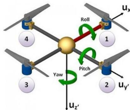
**Gambar 2.1** Pitch Roll Yaw Pada *Quadcopter*
