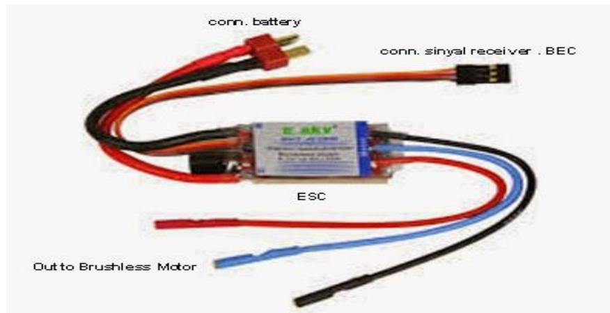
**Gambar 2.6** *Electronic Speed Control (ESC)*
