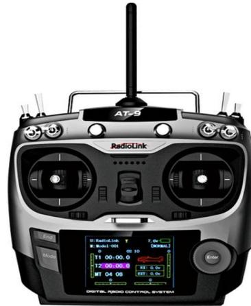
**Gambar 2.3** *Remote Control Radiolink AT-9*
