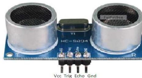
**Gambar 2.7** Modul Sensor ultrasonik HC-SR04
