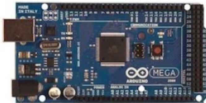
**Gambar2.5**Arduino Mega 2560
