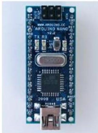
**Gambar 2.9** Arduino Nano 2.x
