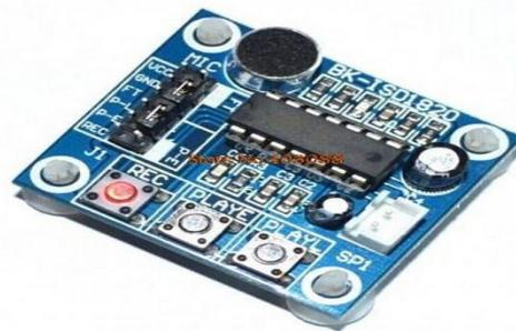
**Gambar 2.8** Modul ISD1820 Voice Recorder
