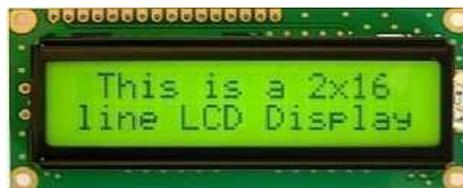
**Gambar 2.12** LCD 16x2
