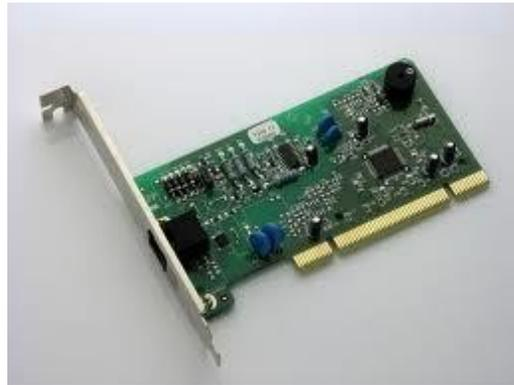
**Gambar 2.5** Internal modem
