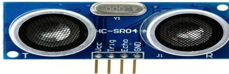
**Gambar 2.15** Sensor Ultrasonik
