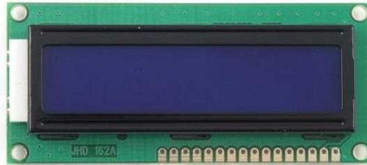
**Gambar 2.8.** Liquid Crystal Display
