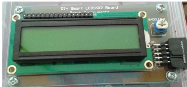
**Gambar 2.4** LCD (*Liquid Cristal Display*)
