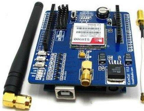
**Gambar 2.6** Tampilan modul GSM SIM900.
