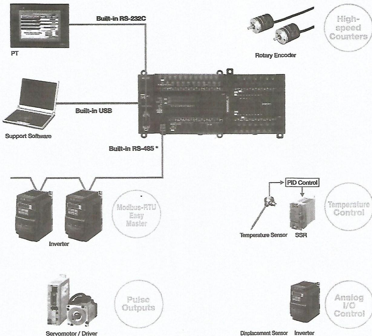
\* Use a built-in RS-485 port of the NaoS1-type CPU Unit or mount an RS-422A/485 Option Board to the Nao-type CPU Unit.
