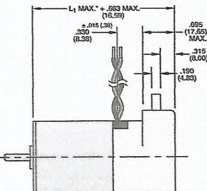
\* The 9237 Motor has a 5mm (.1966) Ø Shaft
