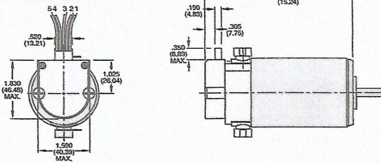
\* The 14207 Motor has a 8mm (.3147) Ø Shaft
