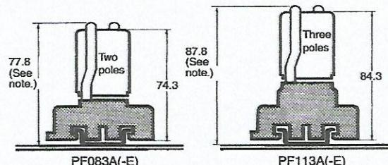
**Note:** PF083A(-E) and PF113A(-E) allow either track or screw mounting.
