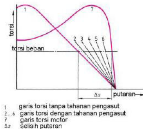
Gambar 2.14 Karakteristik Torsi Motor Slip Ring.
