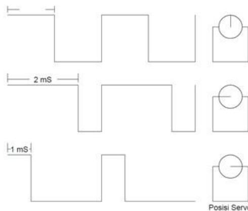
**Gambar 2.8 sinyal pulsa motor DC servo<sup>10</sup>**
