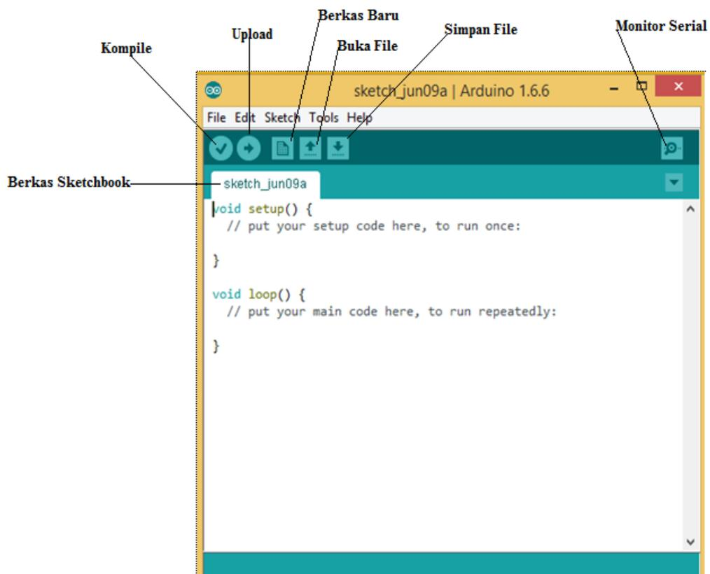
**Gambar 2.4 Menu Ikon IDE Arduino<sup>6</sup>**
