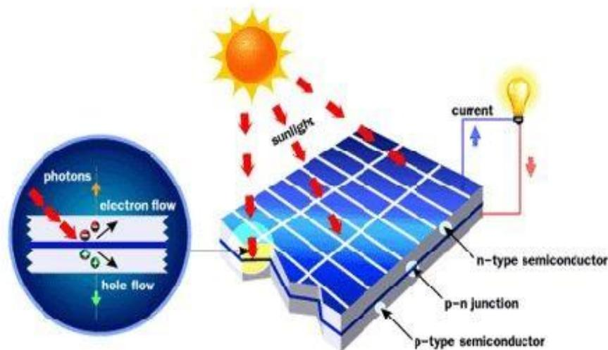
**Gambar 2.1 Prinsip kerja Sel Surya Photovoltaic<sup>1</sup>**
