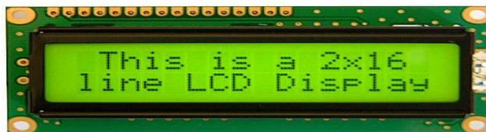
Gambar 2.9 LCD (*Liquid Cristal Display*)<sup>11</sup>
