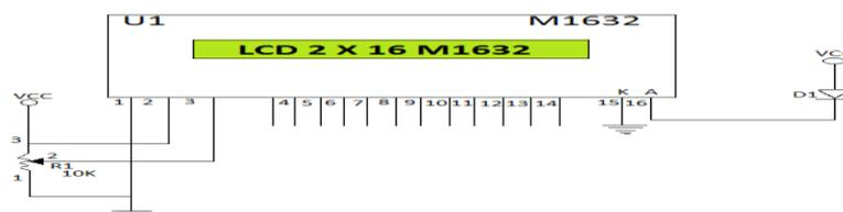
Gambar 2.10 Rangkaian LCD (16x2)<sup>12</sup>
