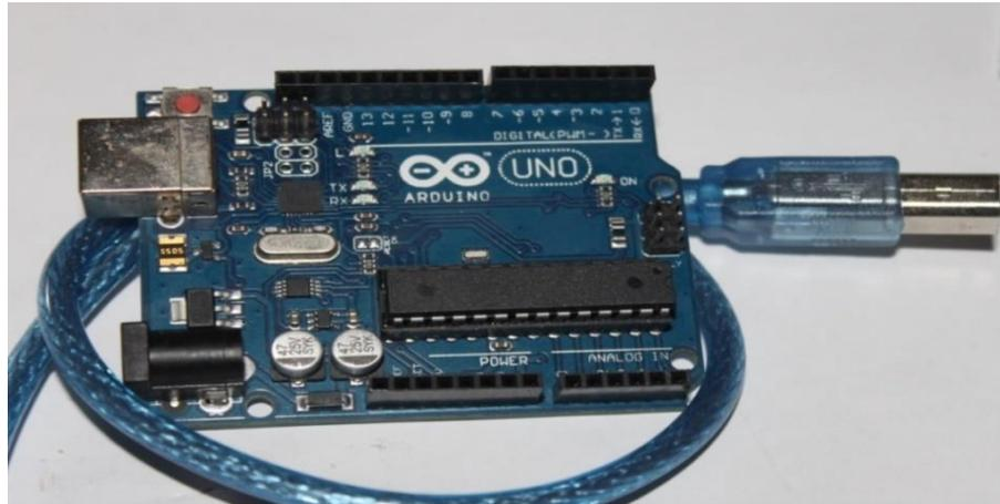
**Gambar 2.2 Arduino Uno<sup>2</sup>**
