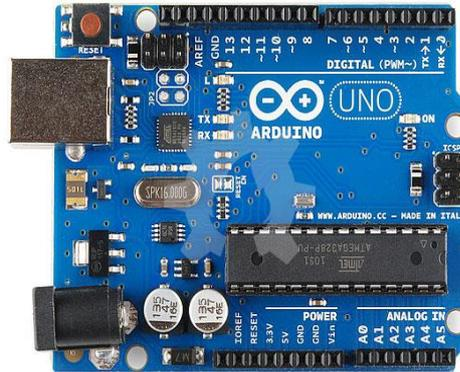
**Gambar 2.5** Papan Arduino Uno
