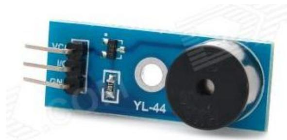
**Gambar 2.13 Modul Buzzer**
