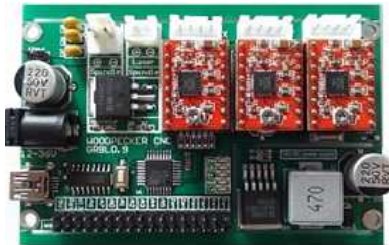
Gambar 2.2 Control Board GRBL 0.9 (Sumber: Sandri, 2017)
