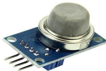
**Gambar 2.6** Sensor Asap (MQ– 02 )
