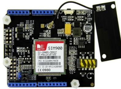
**Gambar 2.7** GSM Arduino Shield
