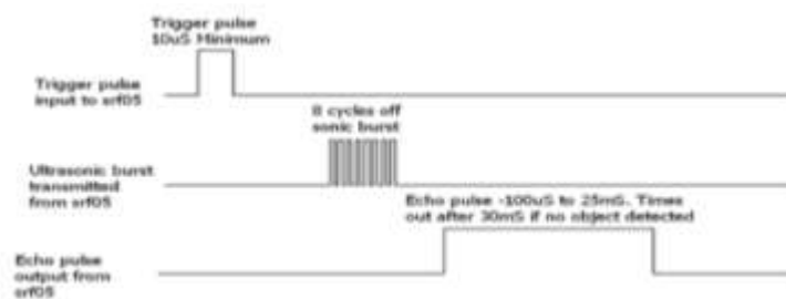
Gambar 2.5 Pulsa Sensor Ultrasonik Mode 1 SRF-05
