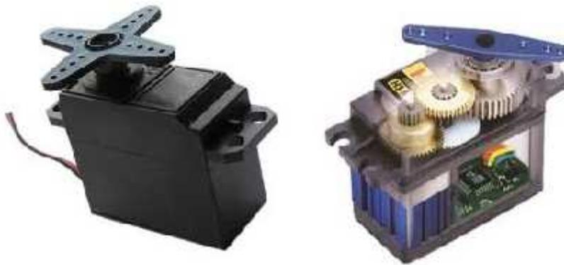
**Gambar 2.7 Bagian motor servo**
