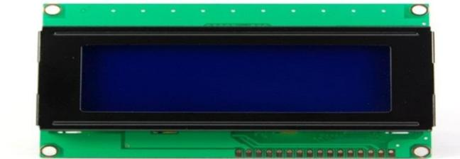
**Gambar 2.8 Liquid Crystal Display (LCD)**
