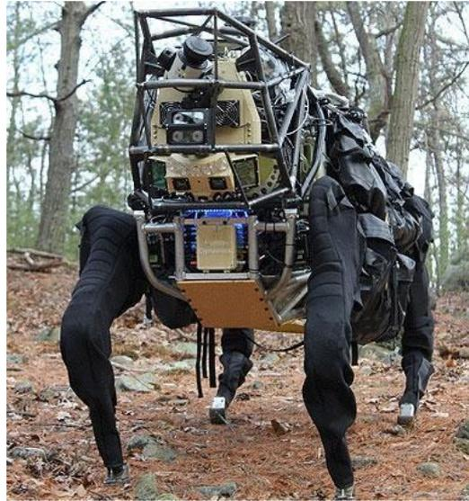
Gambar 2.7 *Semi autonomous legged robot*
