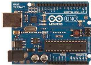
Gambar 2.4 Board Arduino Uno (Sumber: Sano, Adrian. 2012)
