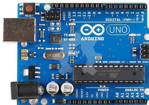
**Gambar 2.19. Papan Arduino Uno**
