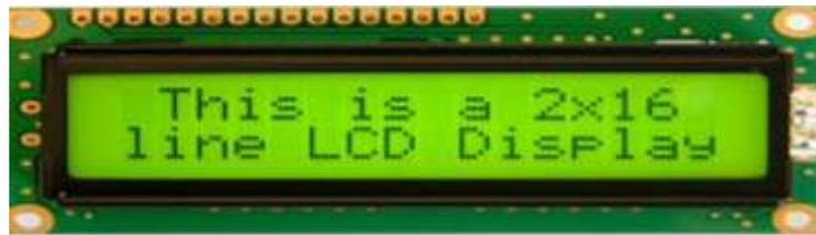
**Gambar 2.17 LCD (Liquid Crystal Display) 16x2**
