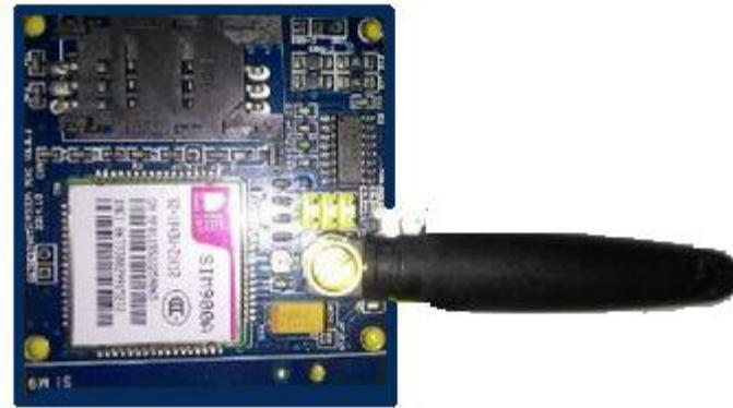
**Gambar 2.4** Tampilan Modul GSM SIM900A.
