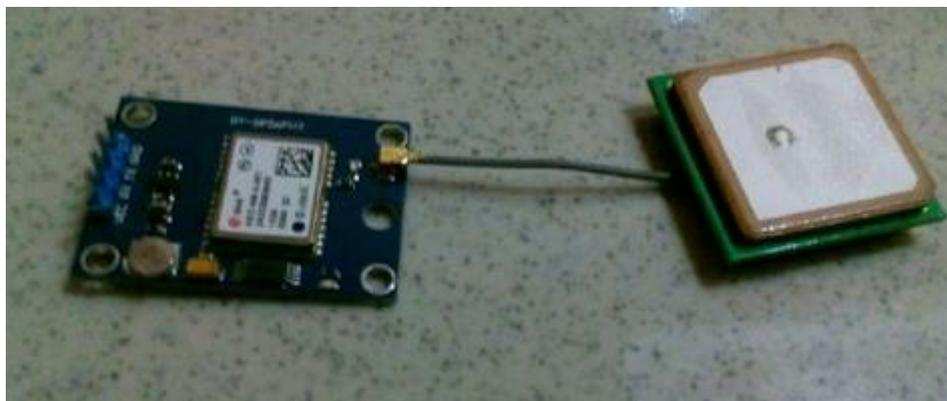
**Gambar 2.12** Modul GPS APM2.5 NEO-6M
