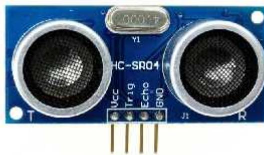
Gambar 2.4 Sensor Ultrasonik HC-SR04
