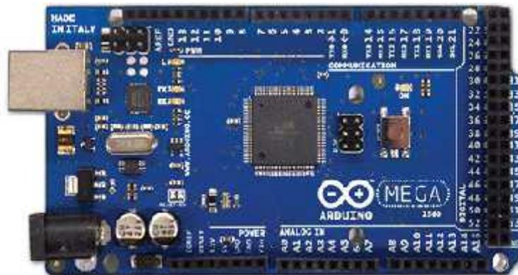
Gambar 2.3 Arduino Mega 2560
