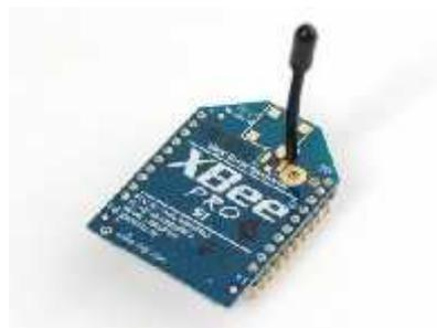
Gambar 2.2 Xbee Series 1[11]
