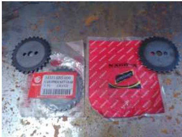
**Gambar 2.10** *Honda Crankshaft Gear*
