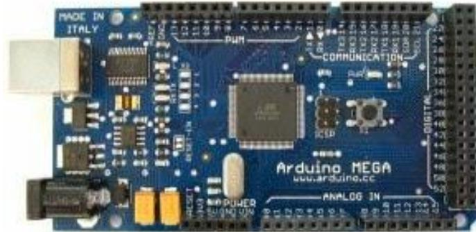
Gambar 2.8 Arduino Mega
