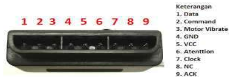
Gambar 2.6 Connector Modul Receiver PS2 Controller
