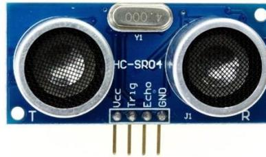
**Gambar 2.12 Sensor Ultrasonik**
