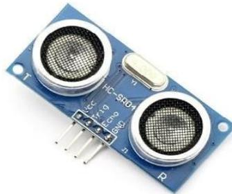
**Gambar 2.5 Sensor Ultrasonik Tipe HC-SR04**
