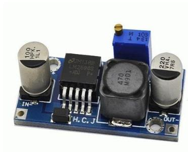
Gambar 2.6 *Adjustable Voltage Regulator*
