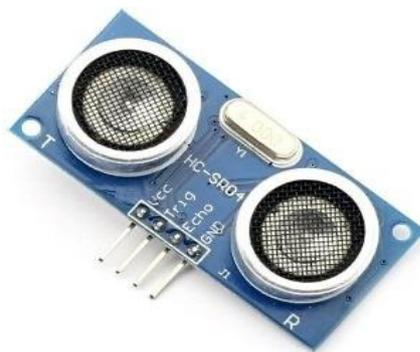
**Gambar 2.16** Sensor Ultrasonik SRF04
