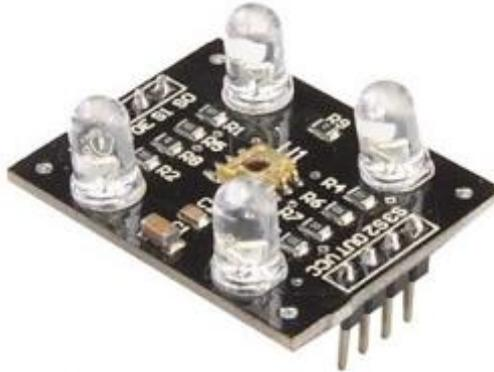
**Gambar 2.15** sensor warna TCS230
