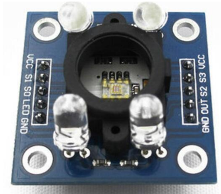
Gambar 2.10 Sensor Warna TCS3200 DT-Sense
