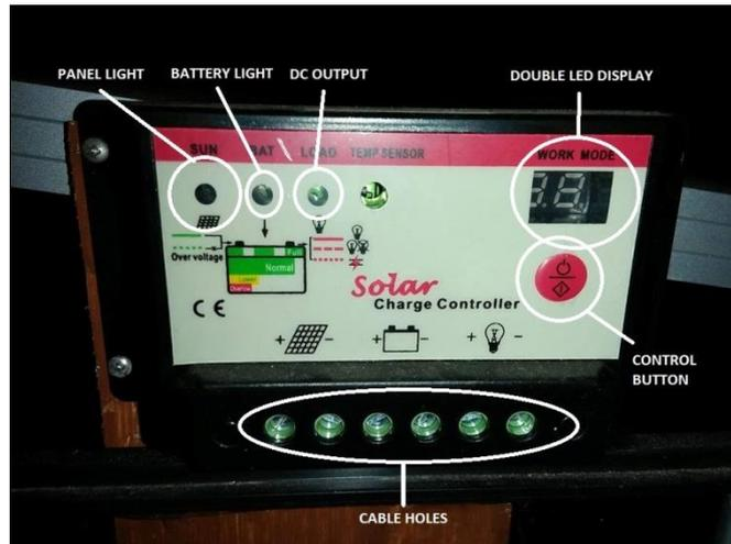
**Gambar 2.19. Solar Charge Controller**
