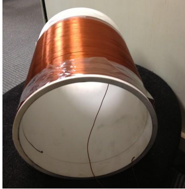
Figure 3. Emitter coil, 10.5 cm radius, 200 turns of magnet wire.
