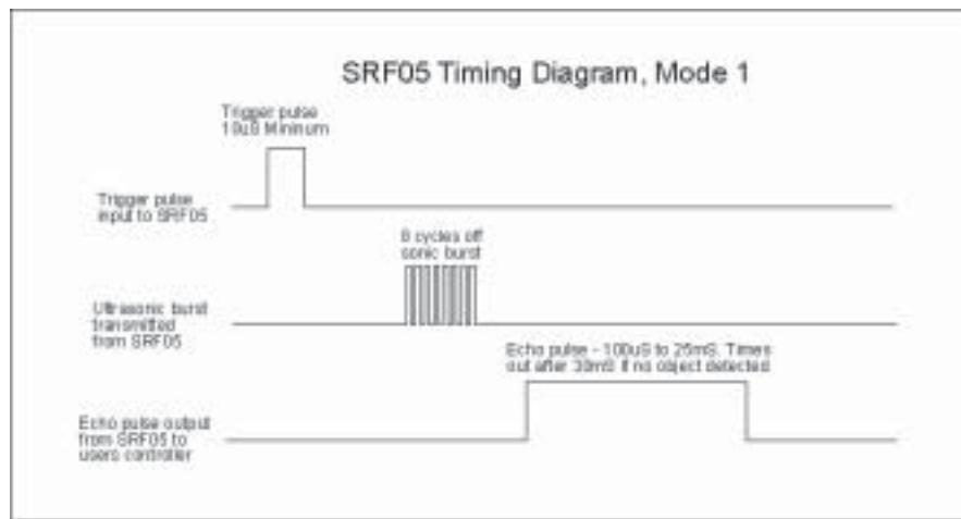
The length of the echo pulse is then divided by 5.8 to give a value in cm, and displayed on the computer screen via the 'debug' command. Note that a word variable, w1, is used for the echo timing, as the echo pulse may be a value greater than 255 (maximum value of a byte variable). Word variables are made up of two byte variables and so have a maximum value of 65535 (in this case w1 is made up of b2 and b3, so they are two byte variables and must not be used anywhere else in the program).
